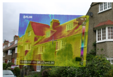
Ground-level thermal image, rectified to overlay a standard photograph to precisely identify problem areas.
